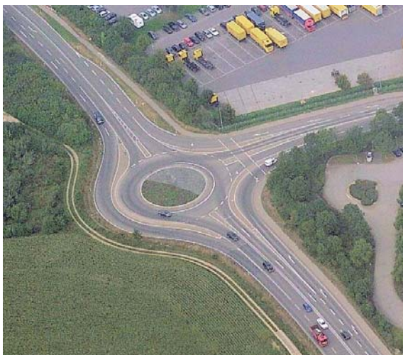
Figure 8 : Rural single-lane roundabout (left side: with three bypass-lanes)
