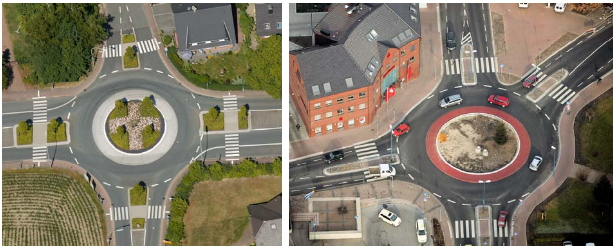
Figure 5 : Compact single-lane urban roundabout (left side: prototype-like design)
