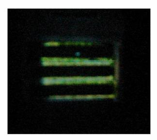
Glowing in the dark. The sample containing Photosynthesis II extracted from spinach is illuminated with X-rays at -260 degrees. The intense beam creates highly reactive species that rest at low temperatures but trigger chemical processes when warmed up to room temperature. These reactions cause the green 'glow'.
