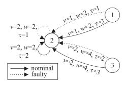
Figure 3: Graph of a timed I/O-automaton
