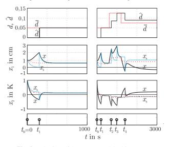
Fig. 4: Behaviour of the process model subject to two different exogenous disturbances
