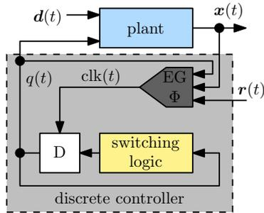
Figure 1: Structure of a discretely controlled system.
