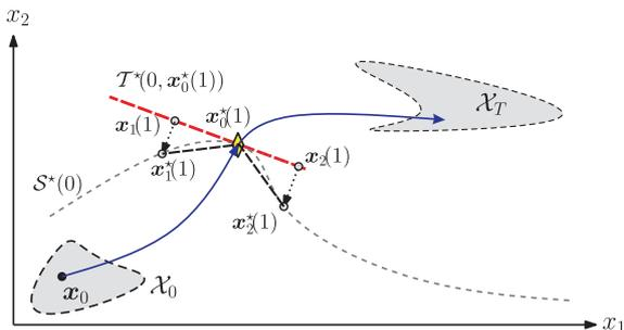
Figure 4: Unfolding of an optimal switching surface.
