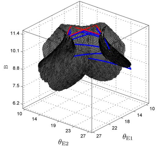
Figure 5: Optimal switching surfaces for the FESTO process. The sample trajectory (blue line) converges to the desired limit cycle (red orbit).
