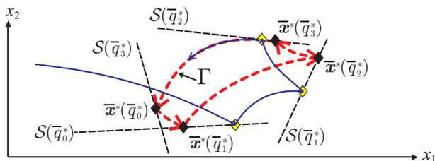
Figure 2: Stabilizing switching planes for a limit cycle  $\Gamma$ .
