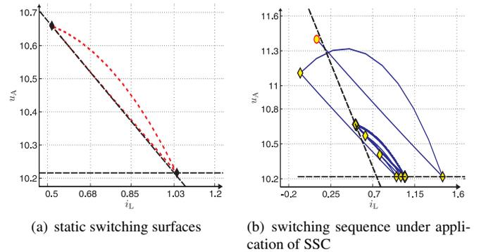
Figure 5: Stabilized limit cycle of a DC-DC Boost converter
