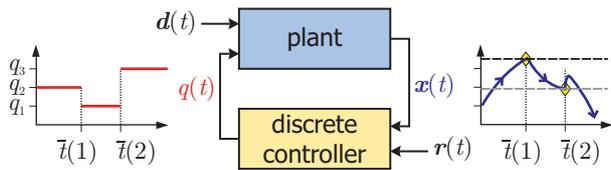
Figure 1: Structure of a discretely controlled continuous system
