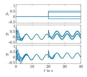
Figure 3: Step disturbances (top), oscillator network without local controller and oscillator network with networked controller which satisfies the internal-model principle.
