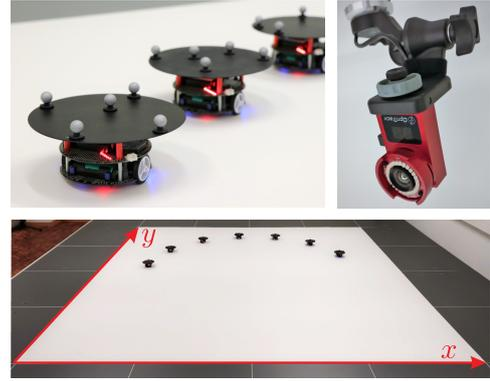
Fig. 4: SAMS with the robots (top left), camera (top right) and the driving surface (bottom)
