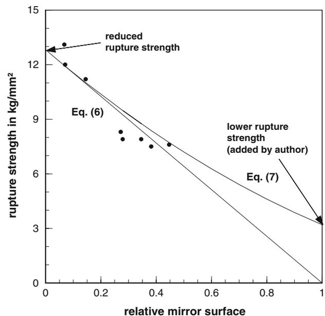
**Fig. 3** Example of a *material curve* according to Smekal's definition. Measurements (at room temperature) taken from Apelt [10]. The *dotted line* is illustrative only. Its calculation is based on the strength values listed in the last line of Table 1
