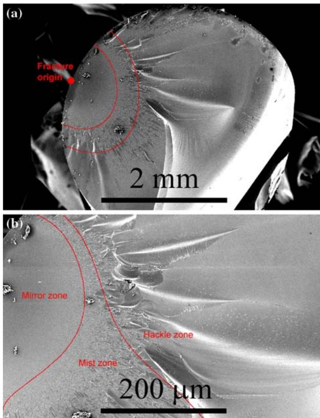
**Fig. 2** Fracture surface of a glass rod broken during a tensile test. **a** General view with fracture origin; **b** topographical features (Photographies: University of Cambridge, Cambridge, UK)
