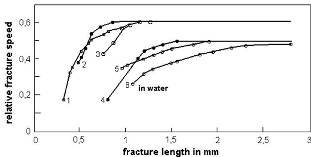
**Fig. 7** Fracture propagation velocities in glasses as functions of loading rate and environment [19]. 1 Quartz glass  $3.45 \text{ kg/mm}^2$ , 2 quartz glass  $4.47 \text{ kg/mm}^3$ , 3 quartz glass  $4.17 \text{ kg/mm}^2$ , 4 optical glass  $2.94 \text{ kg/mm}^2$ , 5 optical glass  $3.25 \text{ kg/mm}^2$ , 6 optical glass  $2.70 \text{ kg/mm}^2$  (in water)
