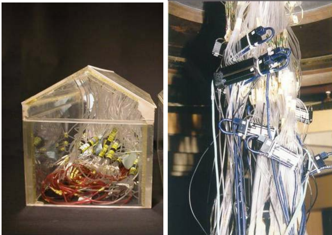
Figure 9: Pressure transducers inside a model (left), or under the wind tunnel turn table (right) (picture left from Benoit Parmentier, WTCB, Belgium)
