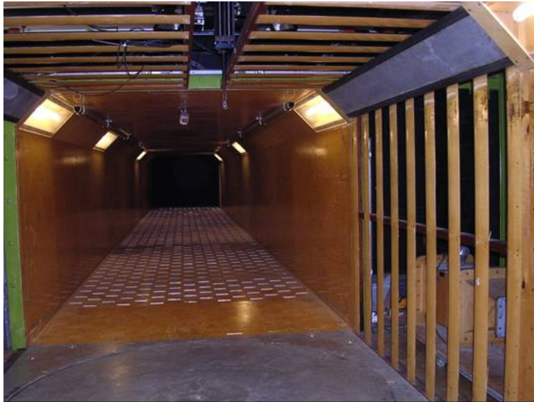
Figure 4: Interior of BRE wind tunnel, with slotted walls at the side and ceiling of the test section.
