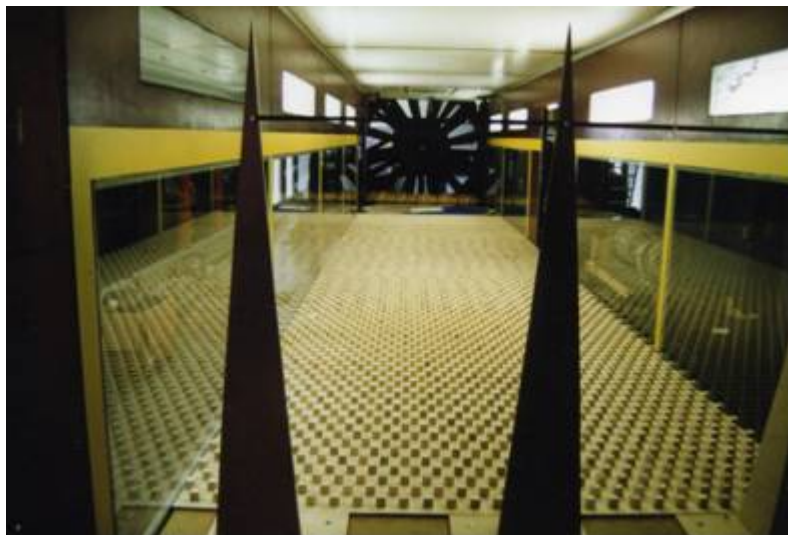
Figure 6: Downstream view of the wind tunnel in Bochum: spires, roughness elements, turn table, fan.
